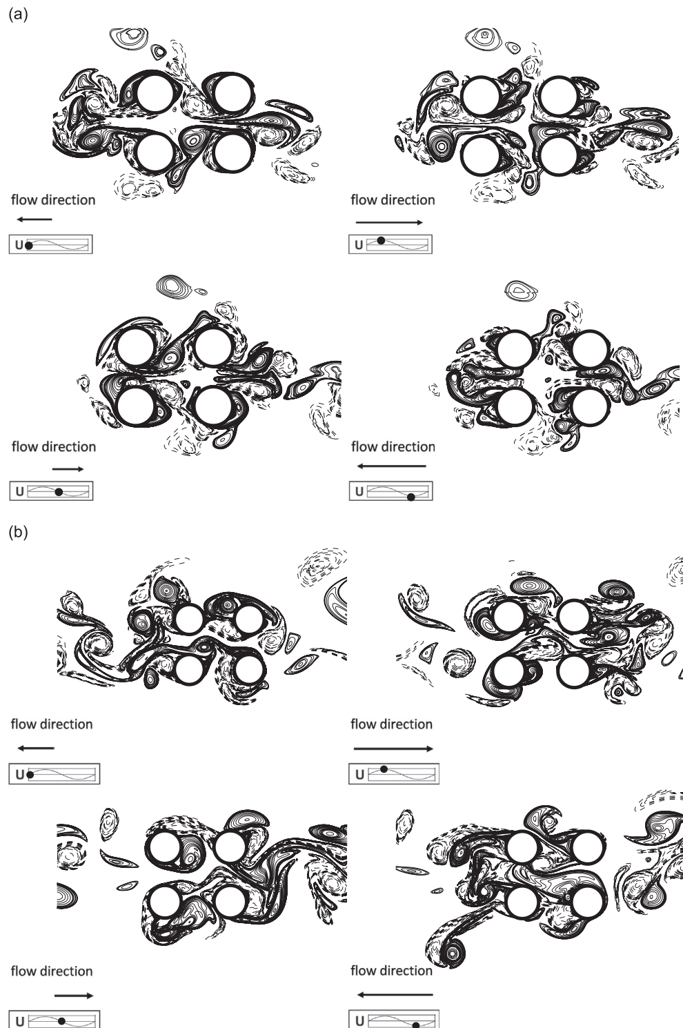
Fig. 7. Snapshots of vorticity contours in the horizontal oscillatory flow interacting with four cylinders during a cycle at (a) KC=5 , (b) KC=10 ; P/D=2 and \beta=50 .
